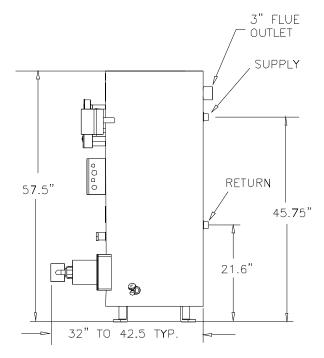
Note: Dimensions subject to change without notice. For ATM boiler, flue is 9 " out the top, 6" if oil burner .
